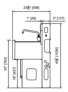
TS (18-9/16"D) & TSF (24"D) Series Three Compartment Sinks (M3) with and without Drainboards
