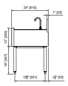
TS (18-9/16"D) & TSF (24"D) Series Three Compartment Sinks (M3) with and without Drainboards
