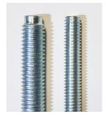
The premium brand on the left and the cheap one is on the right... the premium brand is designed to keep the threads from deforming when you drive the anchor into the drilled hole.
