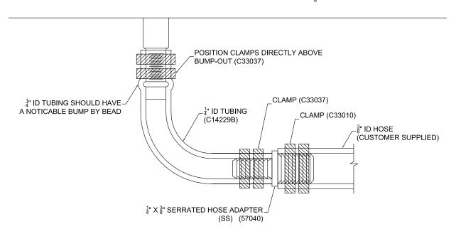
NOTE: An adapter may not be required depending on the size of the soda line being installed by soda provider.
