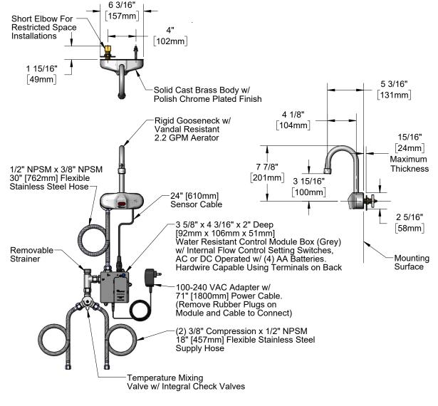
Rough-In Requirement: (2) 1" [25mm] Mounting Holes on 4" [102mm] Centers
