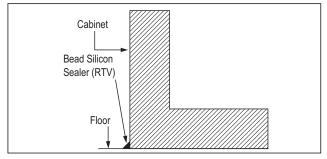
Figure 1. Sealing Cabinet to Floor
