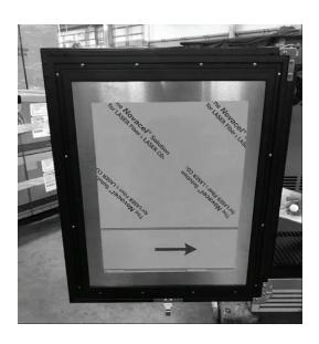
6. Make sure the overlay panel is aligned properly with the door.
