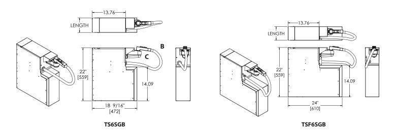
Soda A) manifold; B) hose gun; and C) drip cup NOT included. Shown for clarity only.
