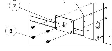
STEP #8: SECURE BOTH CABINETS TOGETHER AT THE BACK WITH (1) 1017862-1 AND (4) 1008781
