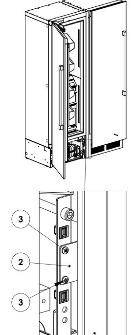
STEP #7: SECURE BOTH CABINETS TOGETHER AT THE TOP WITH (2) 1017862-1 AND (8) M50050-466
