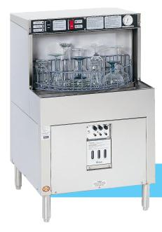
Model PKBR24 Batch Rotary Style glasswasher is easy-to-use and maintain. It has a convenient top-mounted instrument panel. The glassware is washed, sanitized and rinsed in removeable racks that move glasses in batches – saving handling time and broken glassware. Upper and lower spray arms incorporate fan-shaped spray nozzles that clean the entire glass both inside and out.
