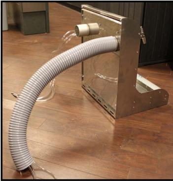
8. Cut a section of hose duct approximately 6" shorter than the length of the beverage leads protruding through the inlets on the back of the dispenser. Note: The hose duct is wire reinforced, so a wire cutter will help ease the cutting process.
