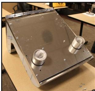
1. Remove screws which secure the back plate to the dispenser.
